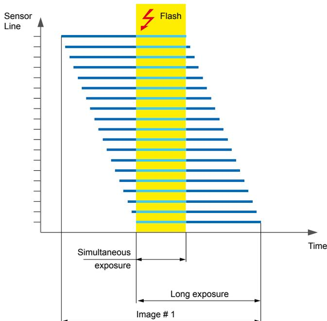
*Compensation for the rolling shutter effect through timely use of flash. The flash must cease at exactly the moment when the exposure of the last row commences and the first row closes.*
