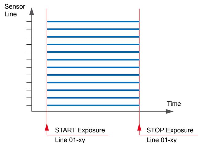
In global shutter mode, the exposure time begins and ends simultaneously for all pixels.
