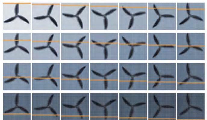
*The yellow line shows the course of the exposure from the first image row to the last. During exposure, then propeller turns four times in total.*
