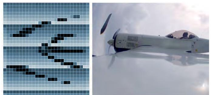
*During the recomposition of the exposed rows into an overall image, the distortion caused by the continuous motion of the propeller is visible due to the row-by-row exposure.*
