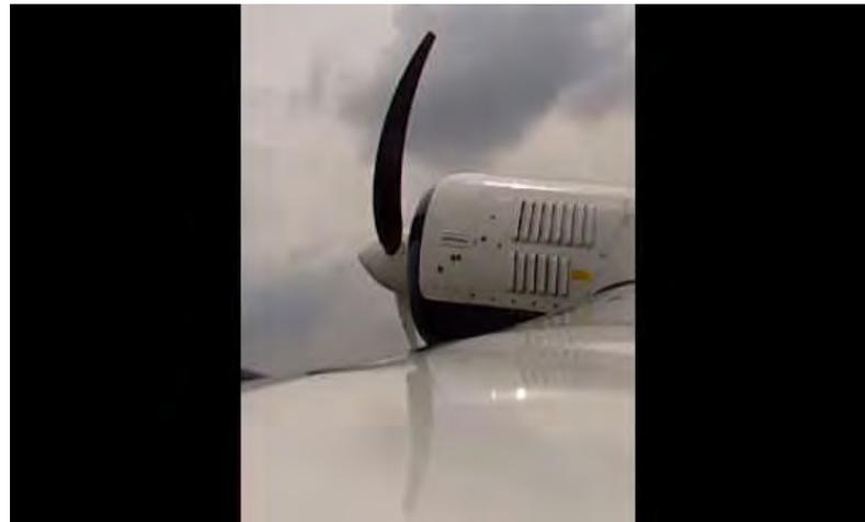
*The rolling shutter effect: The distortion is created by the movement of the vehicle during the exposure of the individual rows.*
