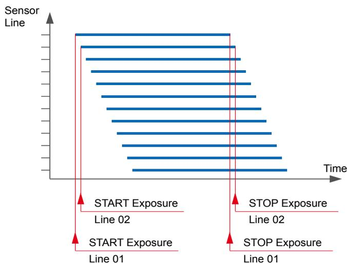
*For the rolling shutter, the exposure time does not begin and end simultaneously, but rather for each individual row respectively: The graphic shows the staggered exposure of the individual rows on the photo.*
