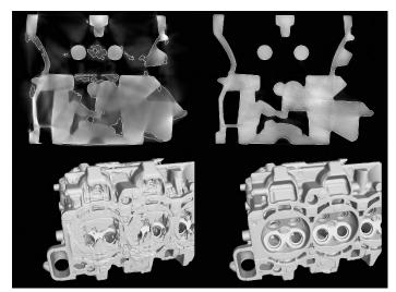
Example for Image Optimization via Software Tools: ScatterFix • Cone-beam CT without (left) and with (right) ScatterFix
