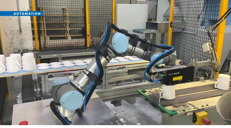
Rotation and positioning data from Matrox Design Assistant X software is communicated to the cobot, directing it to pick and place each teacup.
