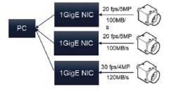
Fig. 1: Three standard BFS-PGE-50S5C cameras connected to a host PC
