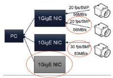
Fig. 2: With Lossless Compression; the "greyed out" GigE NIC is no longer required.
