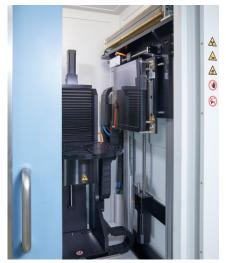
Configuration with flat-panel and line detector
