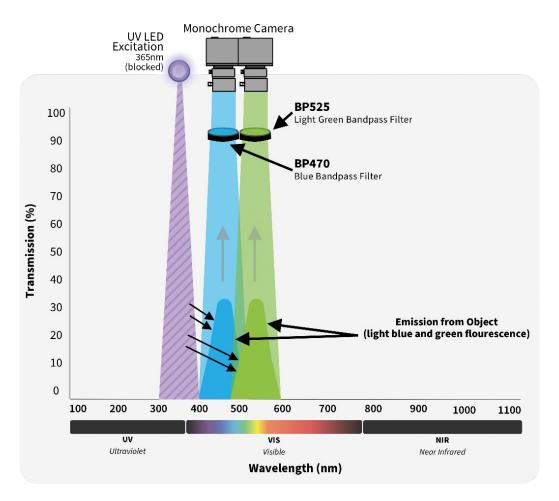
Fig. 1: In machine vision systems, optical filters play an essential role in deciphering the fluorescence emission from the UV light source used for excitation, often overpowering the emission.
