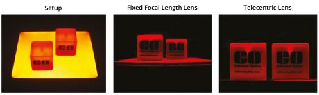
Fig. 1: Middle image: Due to the aperture angle of the fixed focal length lens, the right cube is imaged smaller than the cube of the same size that is closer to the inspection system. Right image: The same scene taken with a telecentric lens. Now both cubes are the same size.
