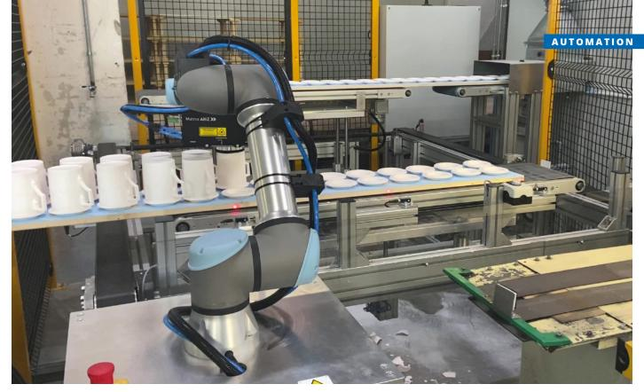
Mounted on the cobot arm, the Matrox AltiZ 3D profile sensor provides high-resolution scans of the pristine white teacups.
