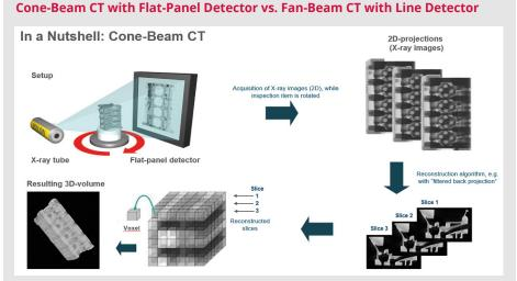
In basic principle, cone-beam CT acquires hundreds of X-ray images from all angles within one complete rotation of the test part, which subsequently get reconstructed via software to a 3D volume.
