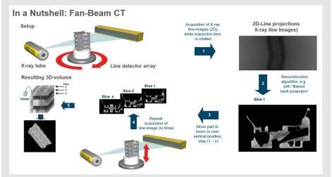
Fan-beam CT is the ultimate for inspecting very large and dense test parts. Here, the test part is scanned pixel layer by pixel layer from all angles. The individual layers get reconstructed via software to a 3D volume. This scanning technique is more time-consuming but virtually free of artifacts.
