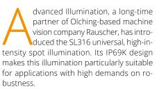
The development of the SL316 was designed to ensure its proper function even after prolonged immersion in liquids, frequent high-pressure steam cleaning and after the use of corrosive cleaning solutions without compromising on the need for an additional protective housing.
