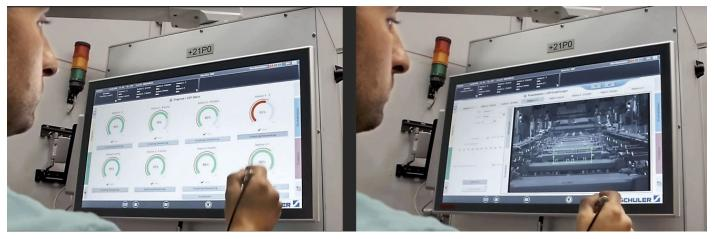
The system detects unexpected causes of faults and stops the press.
