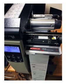
Figure 13: An inline verification system is attached directly to a Zebra® printer to ensure label accuracy while printing.
