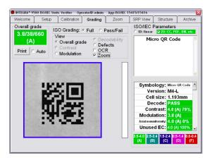
Figure 4: Verification software containing built-in ISO/IEC parameters for grading barcode print quality to standards-based compliance. The QR Code here has achieve "A" grades for the parameters Contrast, Modulation, Axial Nonuniformity, and Unused Error Correction.
