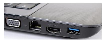
Figure 1. The signature pantone blue USB 3.0 port on a laptop
