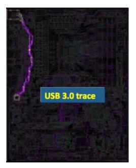
Figure 3. PCB trace between a USB 3.0 port and the physical host controller on a motherboard, highlighted in purple
