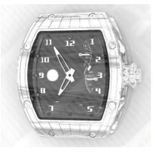
Application Example: Raw image result of the glass window of a watch as seen by a vision system
