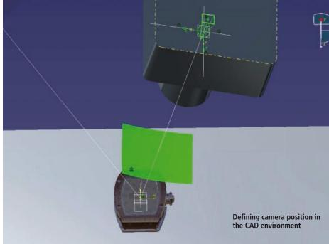
be tested during the simulation in order to find out the optimal system. The simulation result will give the raw image on the sensor - exactly the image that later on will be physically present on the sensor, taking into account the camera parameters.
