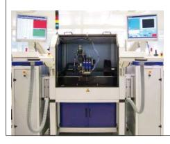
camera. With the images taken by the camera the measuring adapter of the Paneltester can be placed exactly on the contacts. Consequently, possible contact problems as they exist with programmable ICTs are omitted. Furthermore, the camera checks the presence of the components before the test and afterwards it checks the good/bad markings which have been printed on the components.
