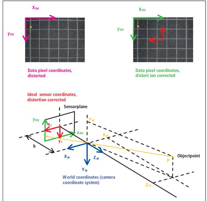
Fig. 3: Coordinate systems for the transformation of world-coordinates to pixel-coordinates in the image data file and the influence of optical distortion
