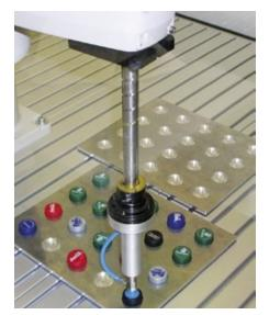
Fig. 1: Pick and place in a plane
