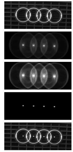
Fig. 4: Hough-transform for overlapping rings a) original image; b) and c) accumulator-images after Hough-transform, raw-image and contrastenhanced; d) accumulator after thresholding; e) overlay of a) and d) showing the centers of the rings as bright spots
