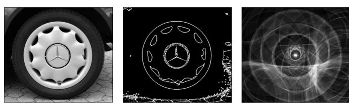
Fig. 3: a) original image; b) boundaries have been isolated and thinned; c) contrast-enhanced version of the accumulator after Hough-transform applied to the boundaries
