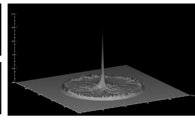
Fig. 2: Houghtransform for a circle a) binary circle in the discrete image plane; b) accumulator-image resulting from Houghtransform; c) accumulator-image, contrast-enhanced; d) central area of the accu mulator with grey-levels as insets; e) 3D-plot of the grey-levels of the accumulator
